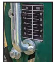
Quick-Adjust Cutting Heights 0.125 - 1.20in (3-30mm)
